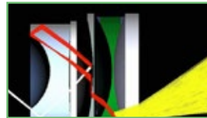
Figure 3: Stray light analysis can help avoid image contrast problems in the final design.
