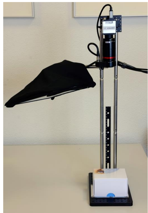
Figure 5: Machine vision setup with a C-mount camera, a 50mm lens and the Optotune focus tunable lens in a front lens configuration.
