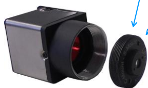
1/2" sensor C-mount camera C- to S-Mount adapter 12mm board lens
